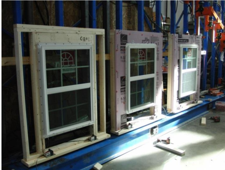
FIGURE 2. LONG-TERM DEFLECTION UNDER SELF-WEIGHT TESTING
