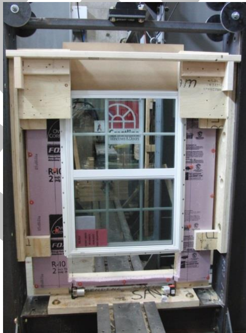
FIGURE 3. STRUCTURAL LOADING – FASTENER/FLANGE CAPACITY
